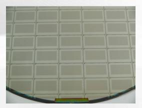
0.25 micron process 8" CMOS wafer - 0.7" HD LCOS
