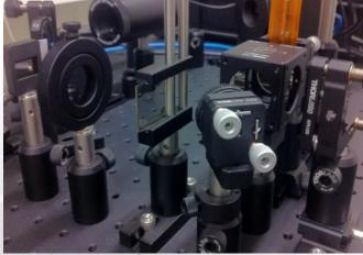
High-speed interferometric measurement system
