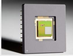
CMOS-based 240x200 piston-type MEMS, courtesy of Fraunhofer IPMS
