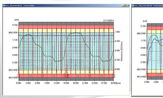
Field gradient and director distribution for a blaze grating, director is parallel to field gradient No overlapped amplitude modulation
