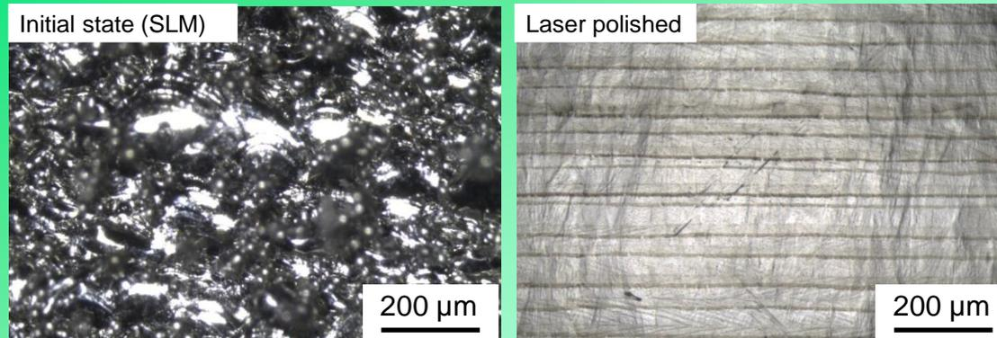
Ra-Reduction: 12-20  $\mu\text{m}$   $\rightarrow$  0.19  $\mu\text{m}$  @ 27 s/cm<sup>2</sup>
