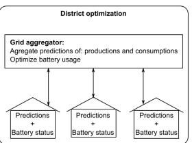
Model predictive control algorithm to optimally use the electric energy flows at building and district level, and lower the consumption and energy bills.
