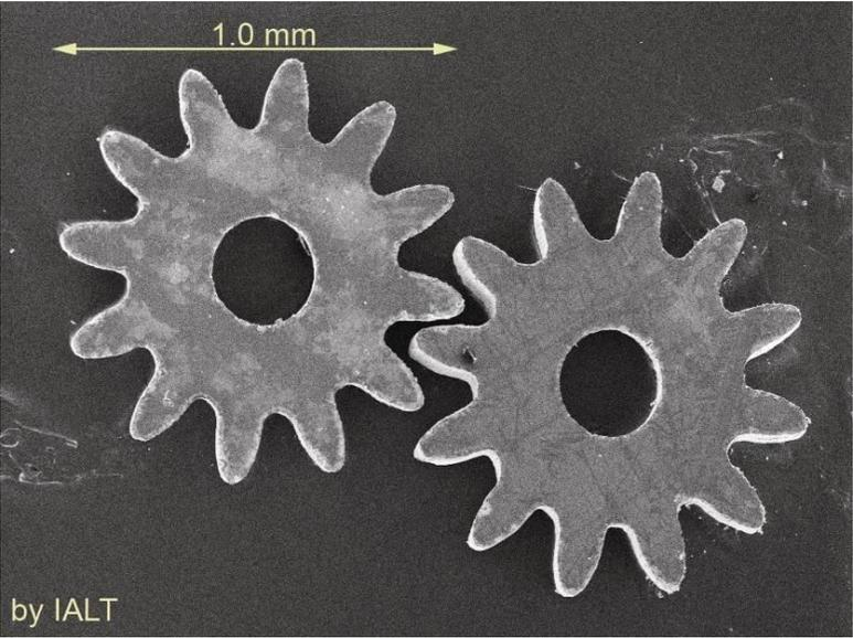
Miniature gears in 50  $\mu\text{m}$  stainless steel foil
