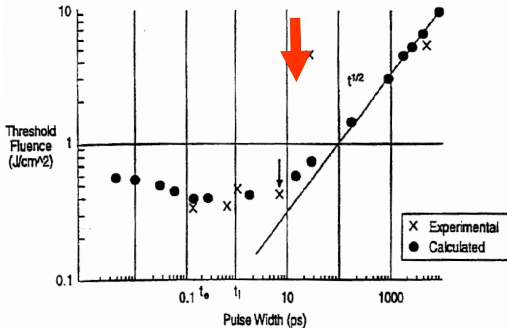
Why? Peak Power required to start ablation is reached at lower pulse energy with shorter pulses
