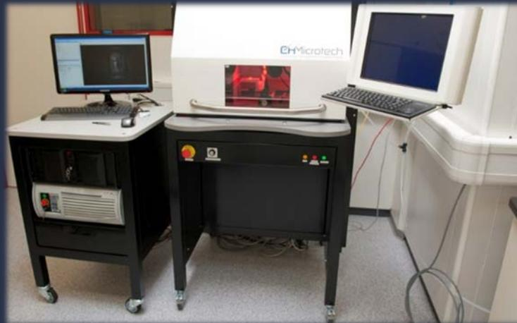
Laser soldering & welding station
