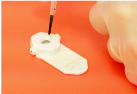
It is possible to measure a liquid metabolic profile by placing a single drop (7 $\mu$ l) into the sensor
