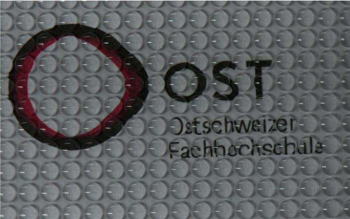
Lens array fabricated by SLE and laser polishing
