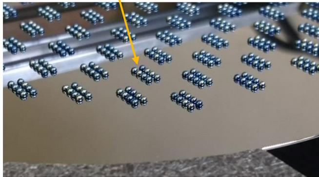
Ball lenses assembled in carrier wafer for IR sensor wafer stack
