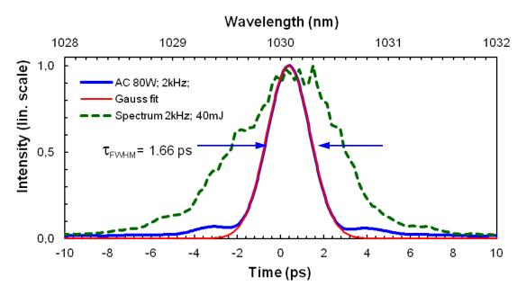
Autocorrelation: 2.4 ps Pulse Duration: 1.7 ps Gauss Fit Bandwidth: 1.1 nm
