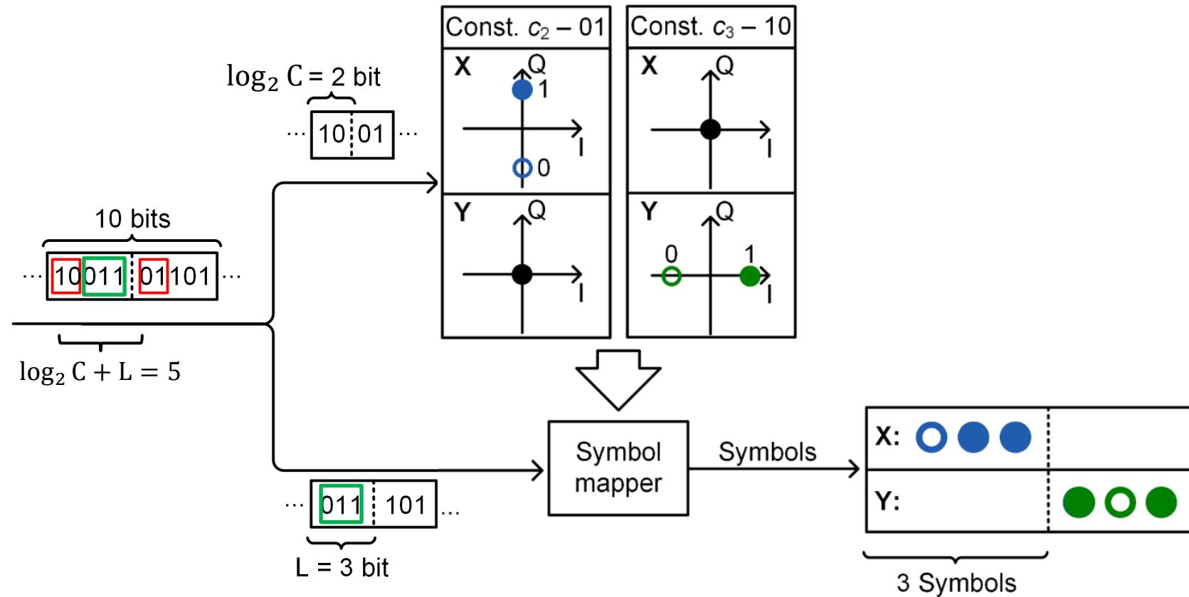
$$\text{Spectral Efficiency } SE = \left[ \frac{\log_2 C}{L} + \log_2 M \right] \cdot \frac{1}{P} \text{ [bit/symbol/Pol]}$$
