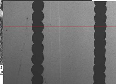
LSM height profile shows a clean trench and sharp edges scribe made at 1064 nm, 30 ps
