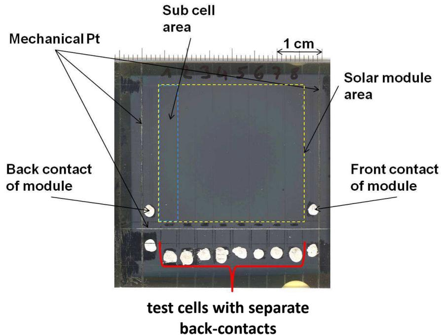
Compare the electrical performance of the single cell with the module performance.
