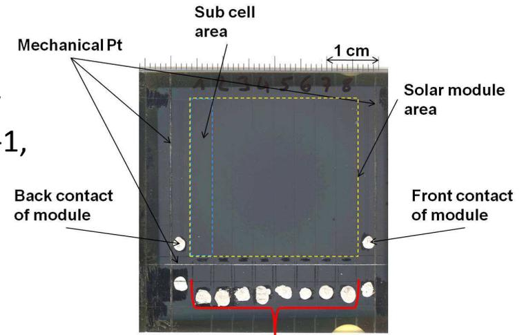
test cells with separate back-contacts
