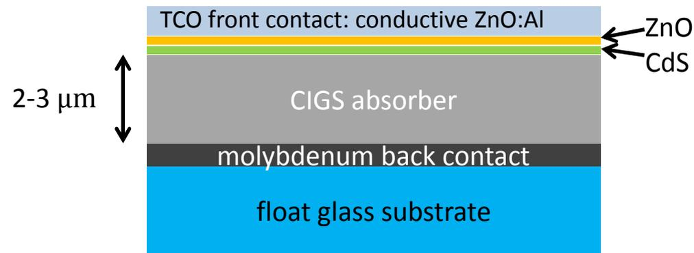
The full multi-layered stack consists of three main functional thin films: a metallic back contact, the absorber material and the transparent front contact.
