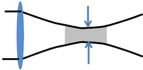
beam  $\varnothing$  4 mm, lens  $f = 40$  mm
