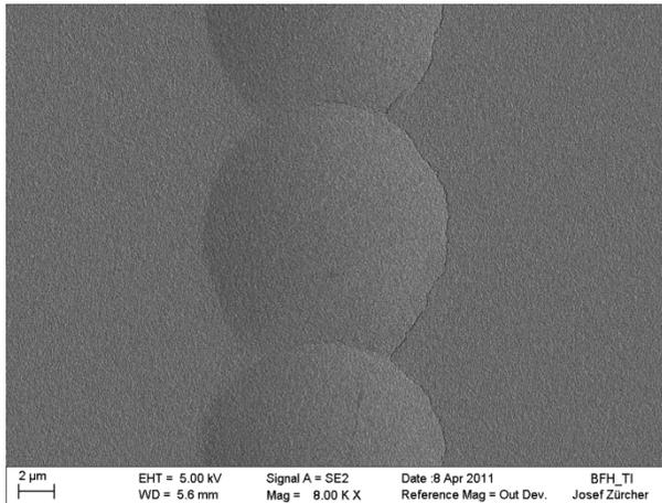
Electron micrograph of a P1 scribe made at 532 nm, 10 ps (below threshold)
