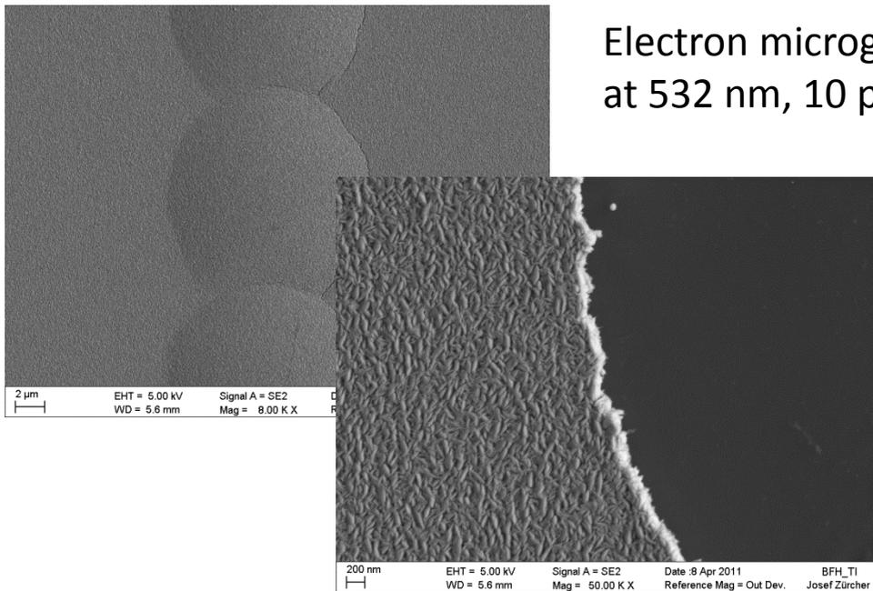
Electron micrograph of a P1 scribe made at 532 nm, 10 ps (below threshold)
