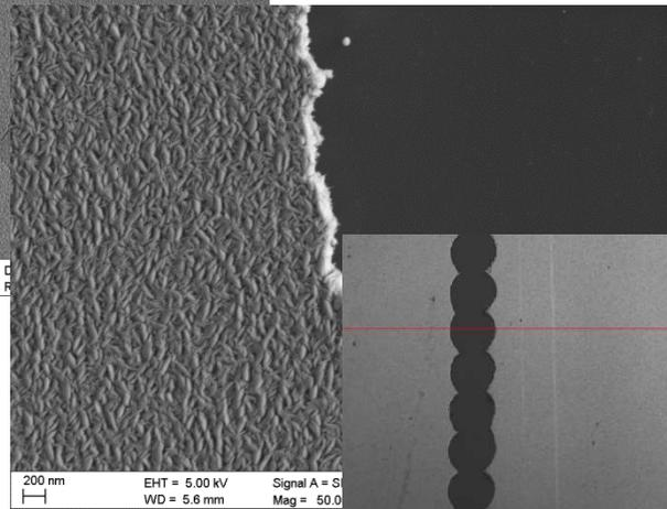
clean rupture of the moly at pulse energies above threshold
