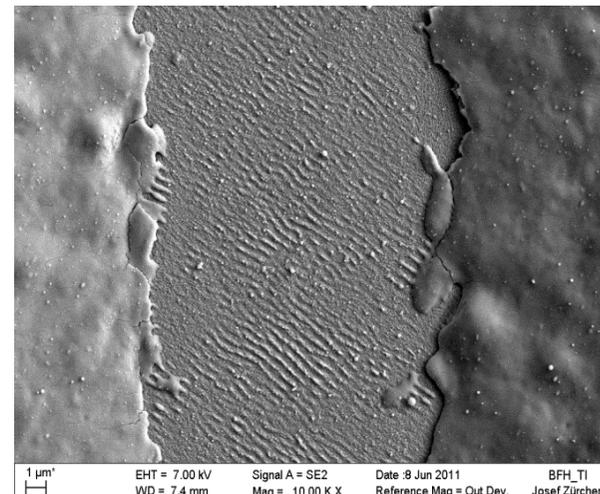
optimized P2 scribe example for 532 nm, 30 ps,  $\omega_0=20 \mu\text{m}$
