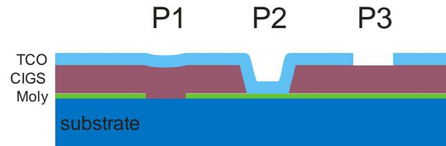
P3 scribe can also remove the whole layer stack down to the Moly
