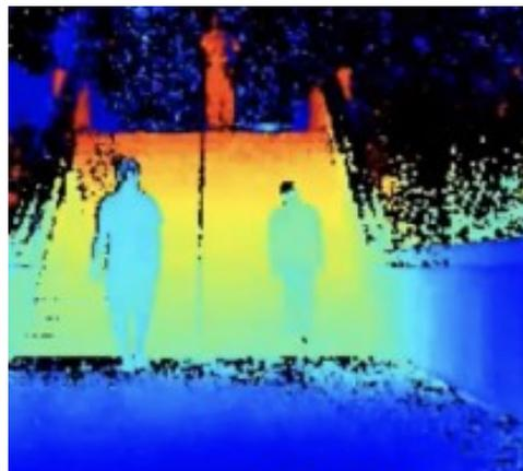
The TOFcam-660 shows all three persons and its ranging capability is not affected by thge sunlight. Even the person with the black clothes is perfectly visible.
