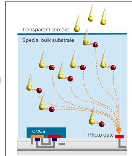
ESPROS' OHC15L backside illuminated CMOS/CCD technology achieves unsurpassed sensitivity in near infrared (NIR)
