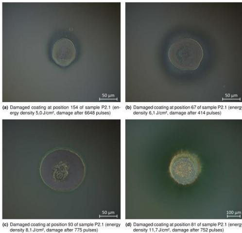
Figure 4: Typical damage morphologies at four spot sites of sample P2.1.
