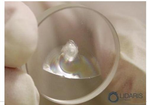
Defect driven damage mode
