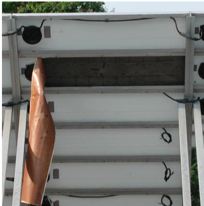
Detachment of first Tedlar layer on the backside
