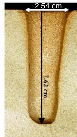
Cross-section of a hole in Sandstone by spallation (3 kW, 62s)
