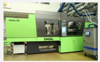
ENGEL injection moulding machine with R2R feeder
