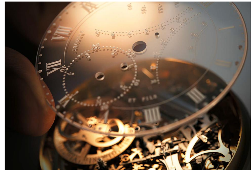
Drilling/Interior marking of Sapphire dials
