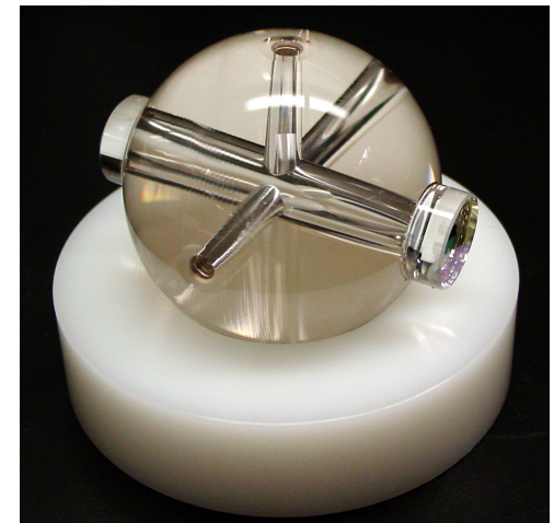
cavity employed for laser stabilization
