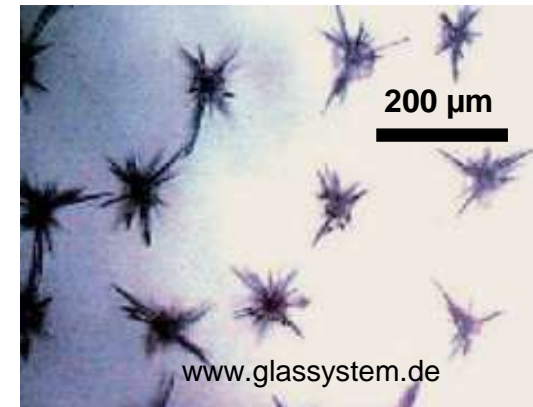
ns-laser, 532nm (thermal process causes microcracks)
