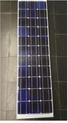
A degradation of 0.11% per year (resulting from the measurement analysis) suggests a performance of the new panel of 45.8 Wp. As compared to the nominal 48 Wp of the data sheet, this is within the tolerance band of  $\pm 10$  %
