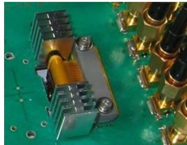
Assembled transceiver module Transceivers realized in collaboration with Intexys Photonics
