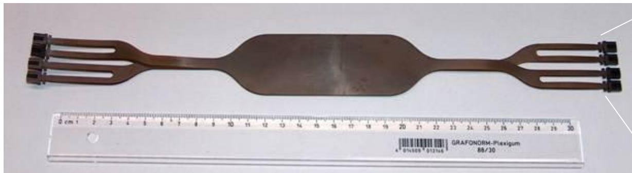
One 'quad L-link', stack of 8 waveguide flex sheets, 192 waveguides, 8 connectors
