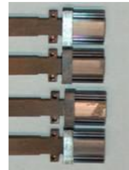
One 'quad L-link', stack of 8 waveguide flex sheets, 192 waveguides, 8 connectors
