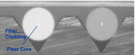
Precise fiber alignment is reached using V-Groove technology, thereby reducing the tolerance chain leading to superior performance.
