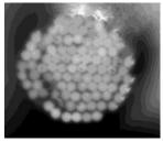
In 1951, H. Moeller applied for a patent on fiber-optic imaging proposing cladding glass or plastic fibers with a transparent low-index material
