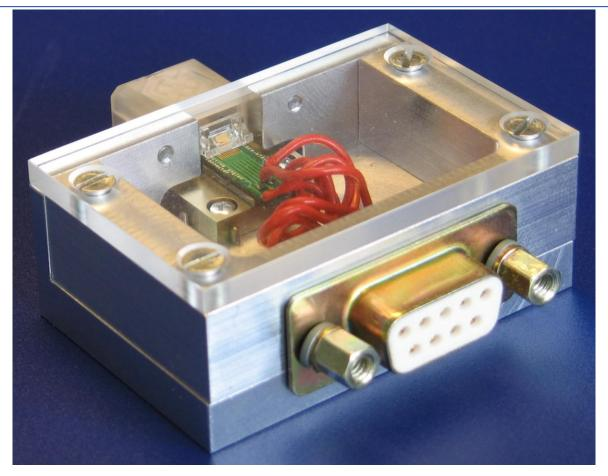
Losses in the range of 3.0 dB at 5 mA were measured (very similar to bare fiber measurement).
