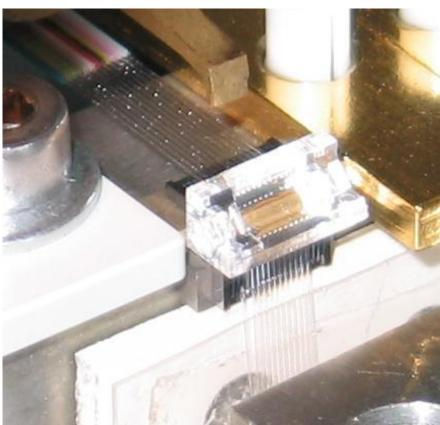
Connectivity solution between FiberBus and FiberBus using subassembly consisting of V-groove substrate and 90° micro-lens array
