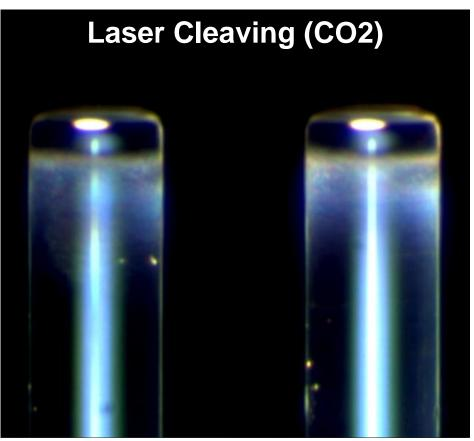
New endface preparation by laser cleaving technology for faster, better and more reliable multi-fiber optical connection.
