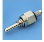
**SMA** (mid 80s) 1/8" (3.125m) metal ferrule not keyed => air gap Losses: 0.5-1dB (still in use in some, industrial applications)
