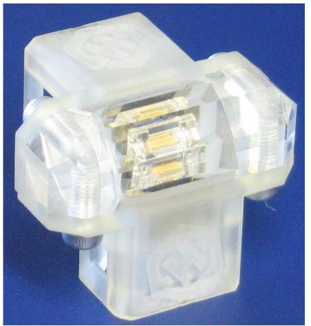
Losses in the range of 1.3 to 2.3 dB at 850 nm were measured (similar to straight solution).
