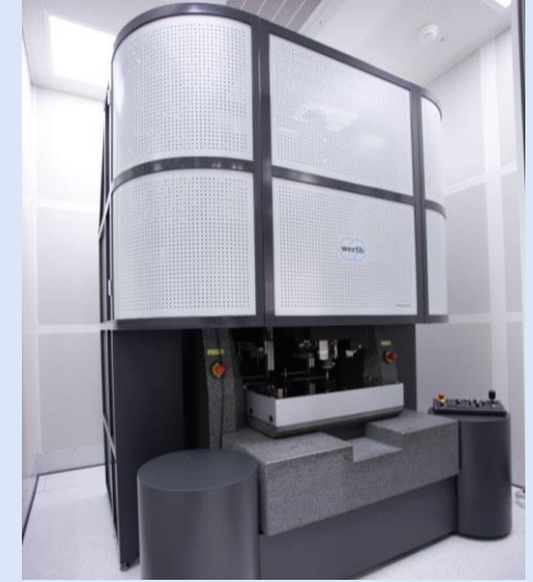
Multisensor coordinate measuring machine WERTH «VideoCheck UA» (measurement uncertainties <math><<0.1\ \mu\text{m}</math>)
