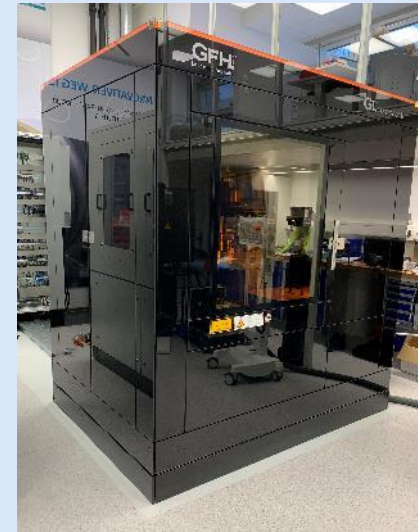
5-axis machining centre with ultra-short pulse laser GFH «GL.compact II» ( \lambda : 1030 / 515 / 343 nm)
