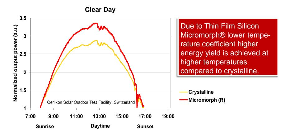
Stabilized modules were used. All data at module level (DC side) to allow comparison of module technologies and exclude inverter influences. Normalized to sunrise.
