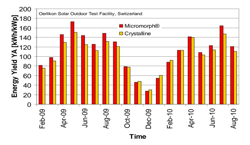
c-Si modules from European manufacturer, best modules in the batch used. All data at module level (DC side) to allow comparison of module technologies and exclude inverter influences
