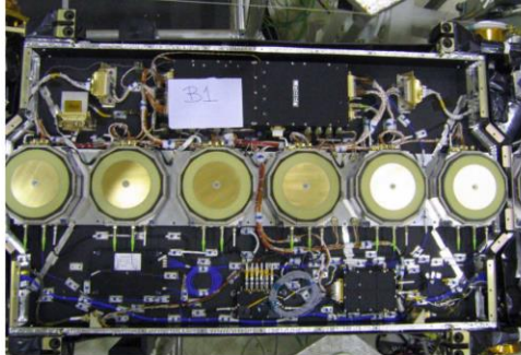
Fig. 7. A MIRAS arm segment with 6 LICEF, 1 CMN, and a fibre-optic 1x8 splitter
