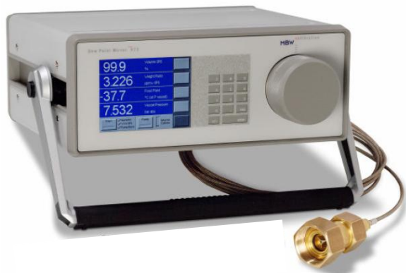
Optical chilled mirror dewpoint meter, MBW
