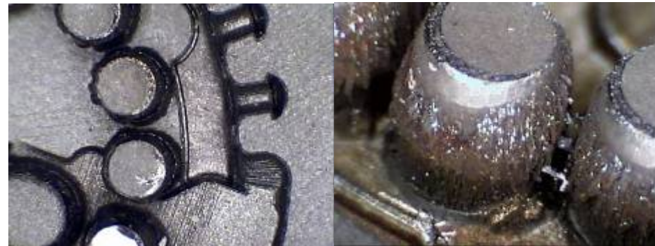
Laser ablation with ns-Laser
