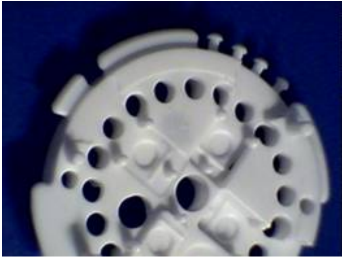
Complex injection moulding part with multiple holes
