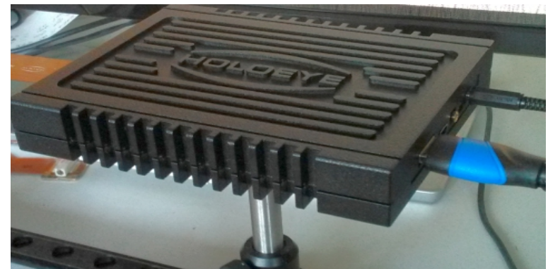
Board in housing with passive cooling
