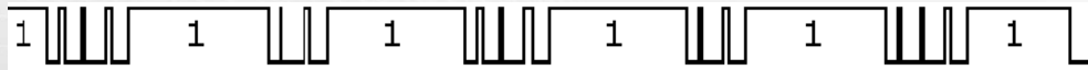
Typical voltage PCM sequence, applied to digital pixel (field inversion ignored for simplicity)
