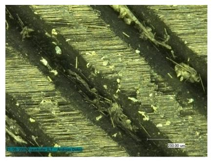
t<sub>Pulse</sub> = 100 ns Rep.-rate: 100 kHz Pulse energy: 50μJ V<sub>Scan</sub>: 1m/s Layer Thickness: 20 μm
