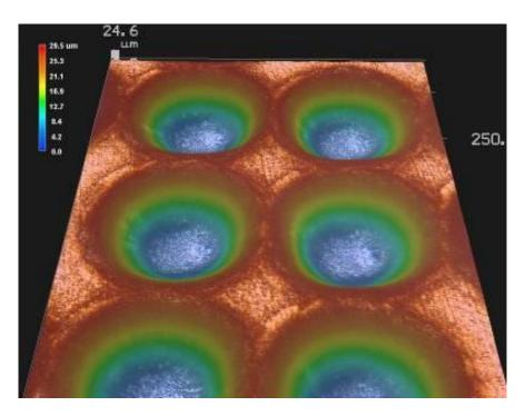
Surface quality After Laser ablation: R<sub>a</sub>= 300nm After Laser polishing: R<sub>a</sub>= 100nm
