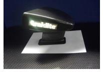
OLED integrated into rear view mirror composite 24h of Le Mans Race
