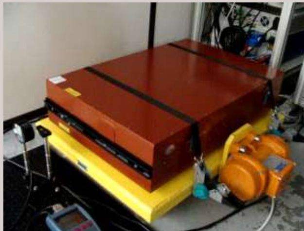
24 HOURS 3g VIBRATION TESTING ON A 1mJ LASER (s-Pulse HP)
