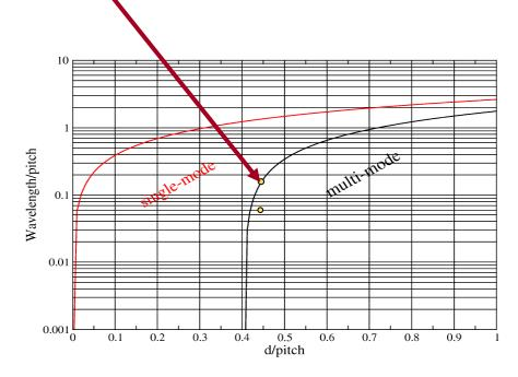
Figure 6: Cut-off phase-diagram
