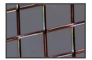
Lower resistance than ITO – Ohmic loss decreased when coming from a small cell to a large module
