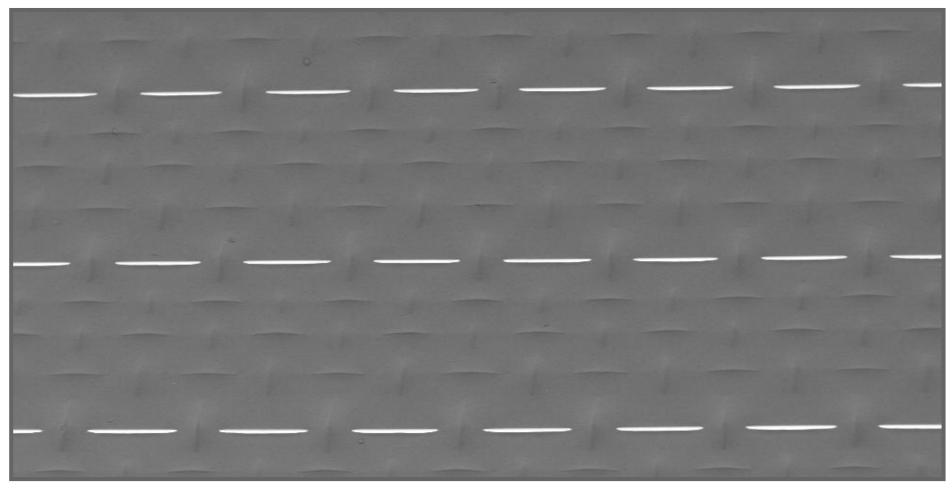
Roughness between hills (thread) and valleys (covered holes) is in the range 5-10 µm
