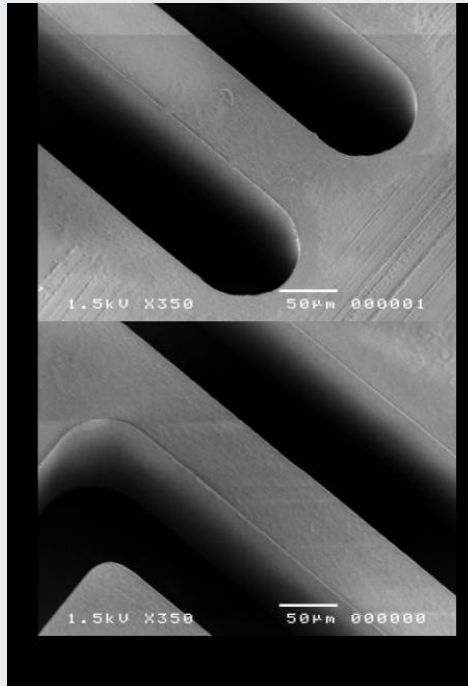
Milling - Sapphire 200 micron wide slot 500 micron deep
