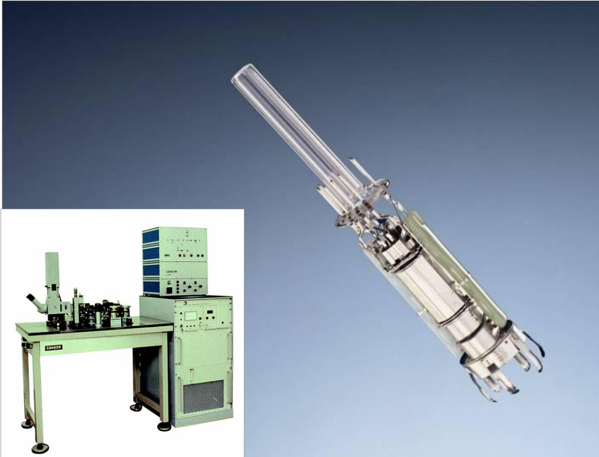
Machine for welding of cathodes for television tubes
