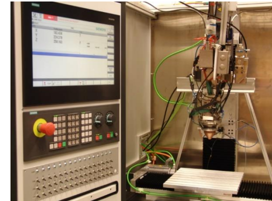
3 axes test setup with Sinumerik 840D sl and Precitec Head and IDM System
