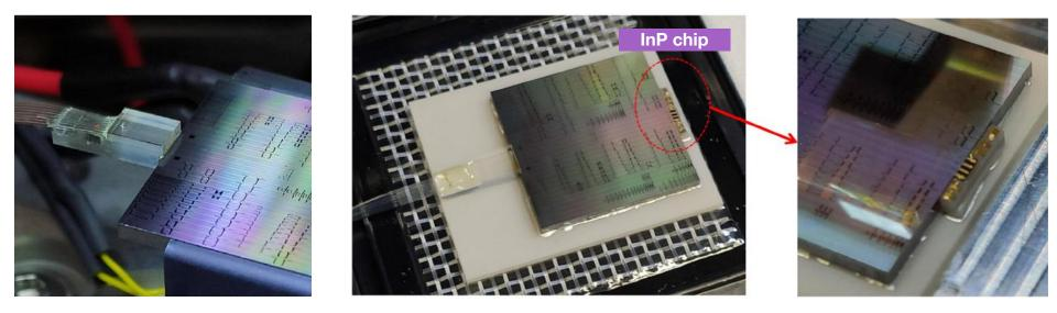
Fiber Array to SiN waveguides
