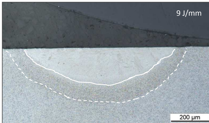
Regular penetration and cross section of a spot applied by a pulsed laser, spot size ~ 800μm
